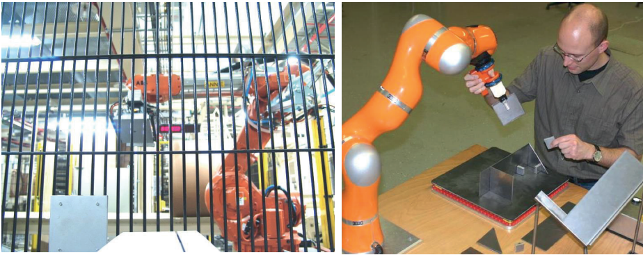
Figure 5 Production environment of industrial robots (left) and cobots (right)
